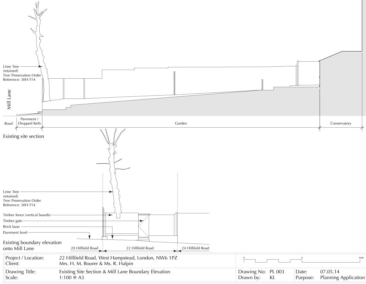
This drawing forms part of a set of Planning Application drawings. It is not intended for Building Control or Construction purposes. Do not scale off this drawing. If in doubt, please ask.
