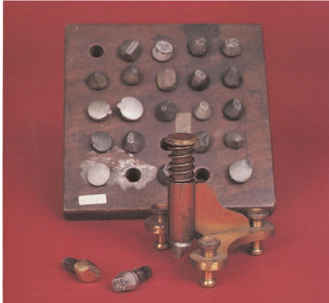
Engraver's spring-punch with a selection of tree and vegetation stamps (page 33)
