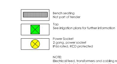
Electrical feed, transformers and cabling requirements to be contractor's designed and approved by electrical engineer.
