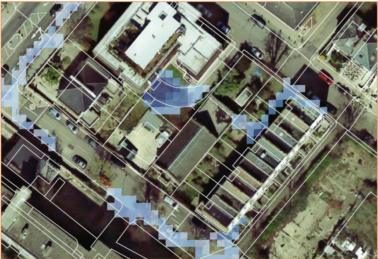
Figure 8: 1:100 year pluvial flood depth mapping (Source: EA)
