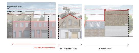
The proposal is not a 'roof', but a new storey and **increase in height of 50%**
