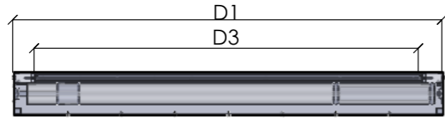
Plan Section FS240 Fire Curtain
