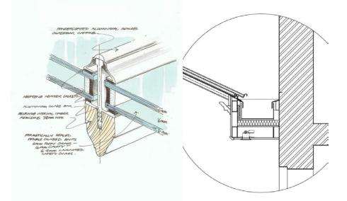
Note: The head of the glazing bars will bear onto a matching profile timber bearer bolted into the existing brickwork. Bolts will be drilled into the mortar perpends.
