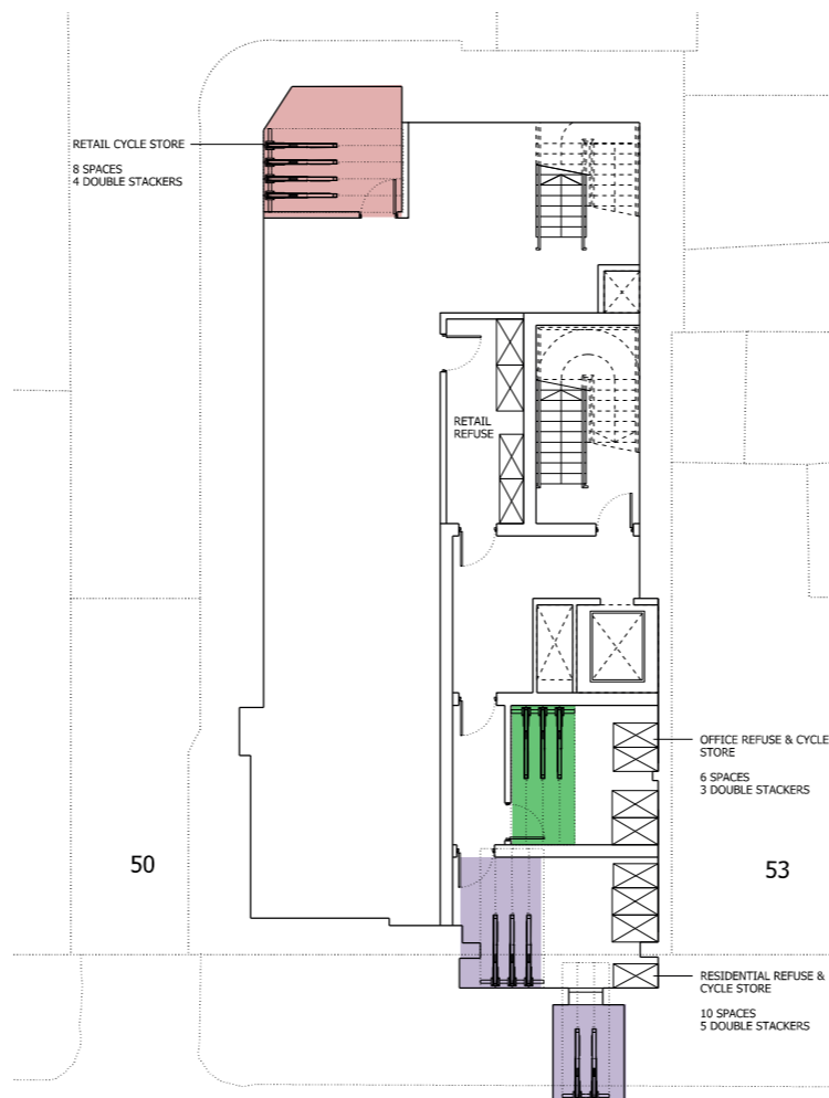
Fig: 3.1 Proposed Basement Plan - indicating cycle storage (double stackers) for each land use
