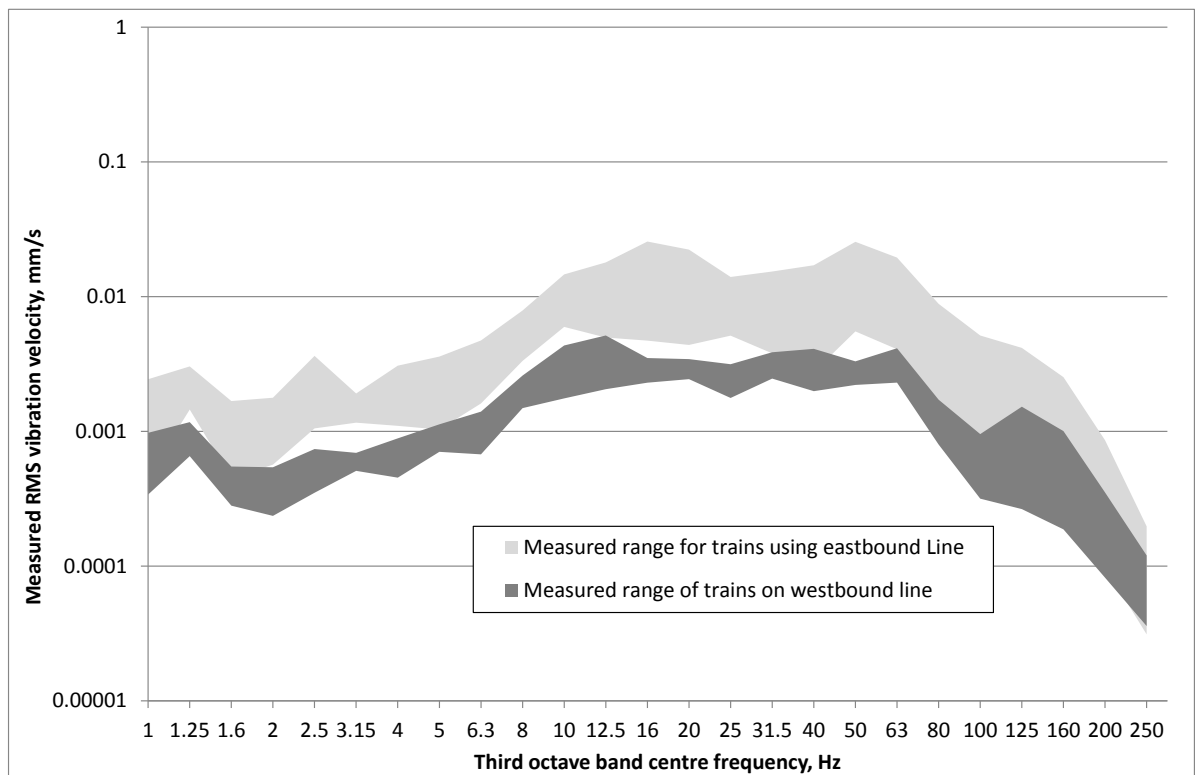
Figure 6 Measured RMS vibration velocity at location 2
