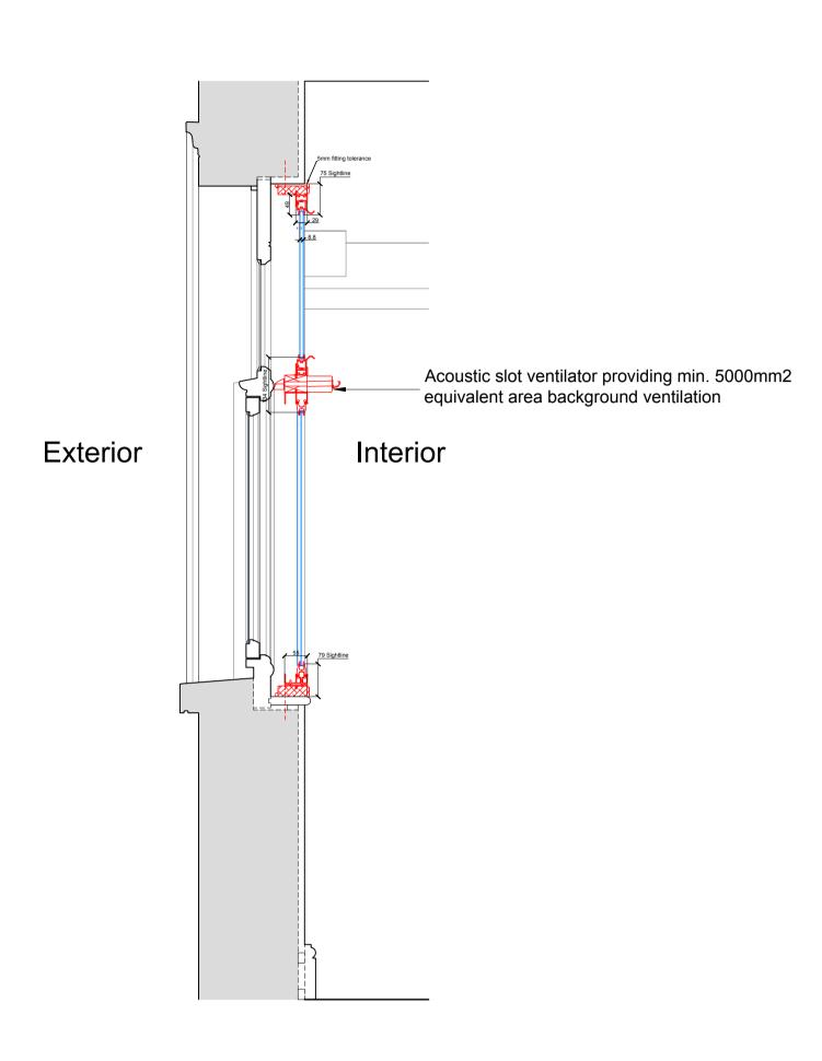
Acoustic slot ventilators to be Greenwood 5000EA with 1 acoustic module fitted to the room side to providie min. 5000mm2 and to 39dB(A)
