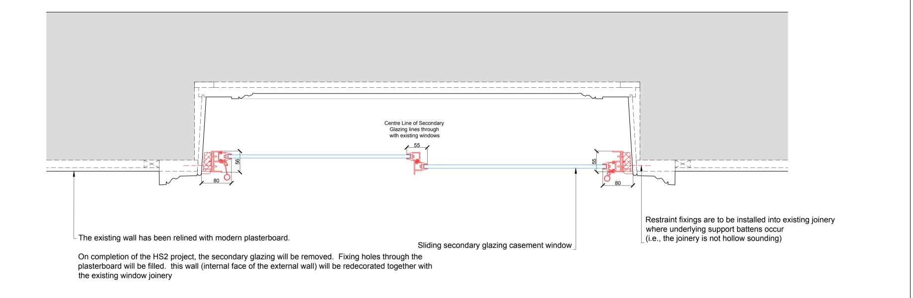
Slot ventilator providing 5000mm2 of equivalent
