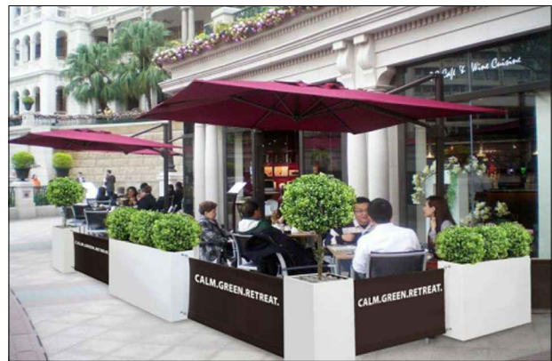
Typical image trough planter screen system with Buxum hedging, 1200mm to top of hedging, with canvas banners at equal length enclosing the tables chairs
