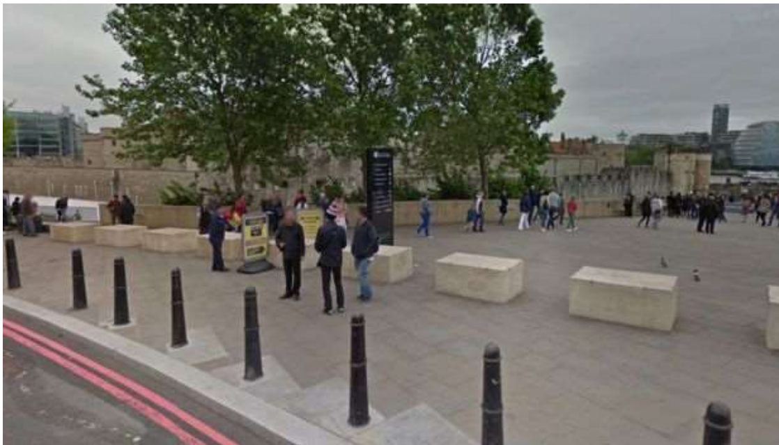
Indicative Concrete Vehicle Block Protection
