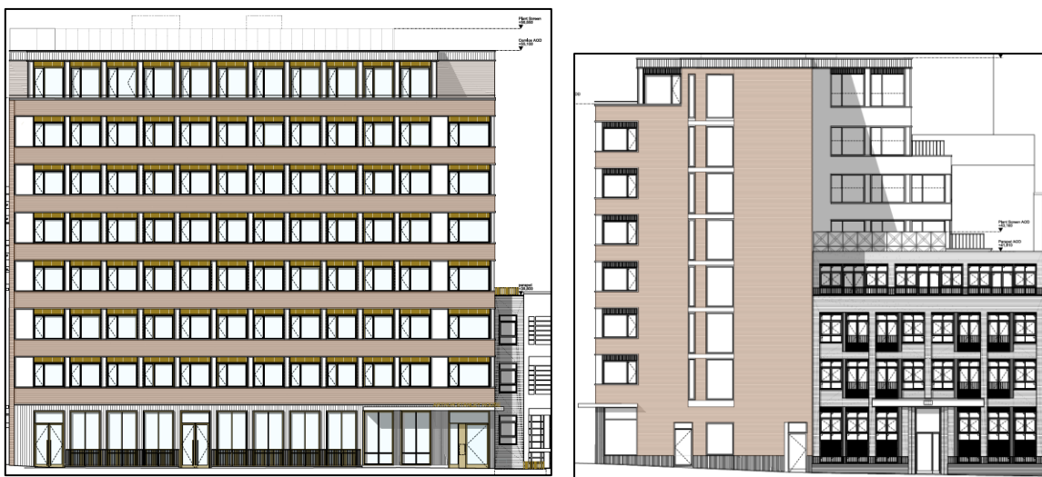
Figure 3: Proposed Development Elevations. Southeast (left) shows the façade of the commercial space, Northeast (right) shows the façade of the residential space
