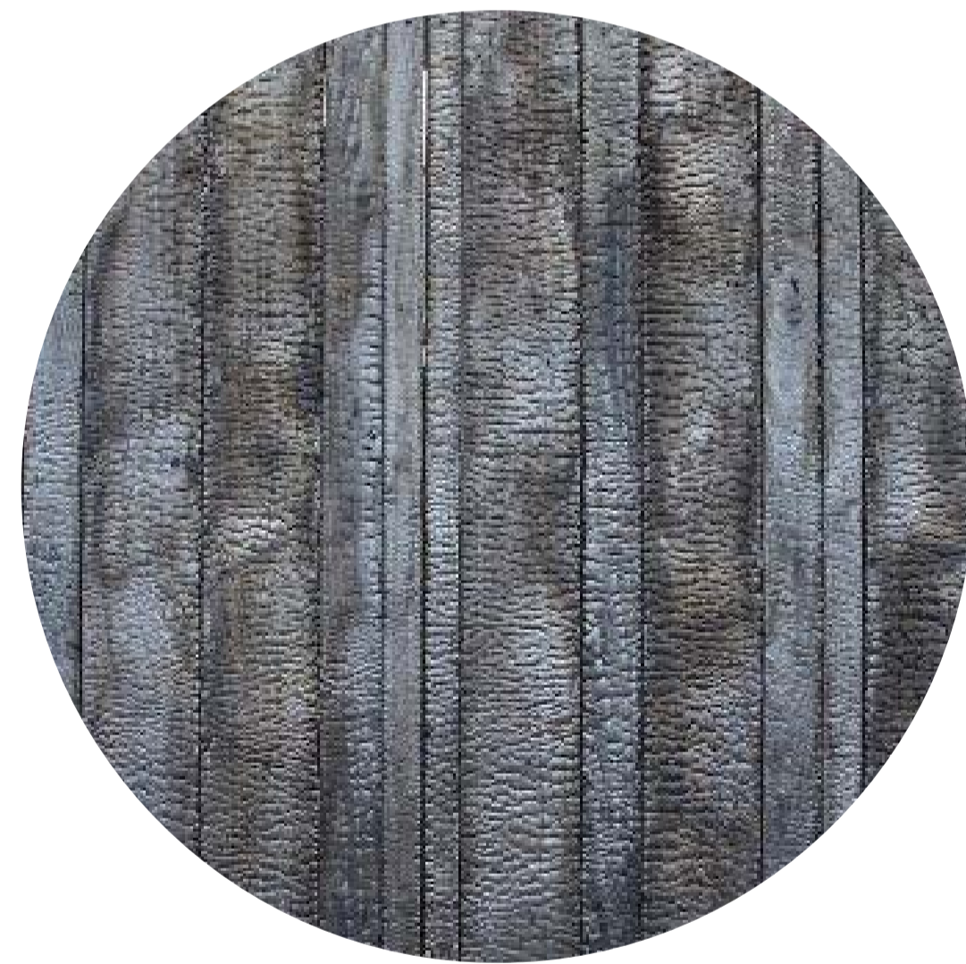
Charred Larch Cladding Location - Block A Balcony Linings / Decking Supplier - Shou Sugi Ban or similar
