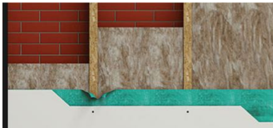
5. Knauf thermoshell solid wall insulation with membrane (anti interstitial condensation)
