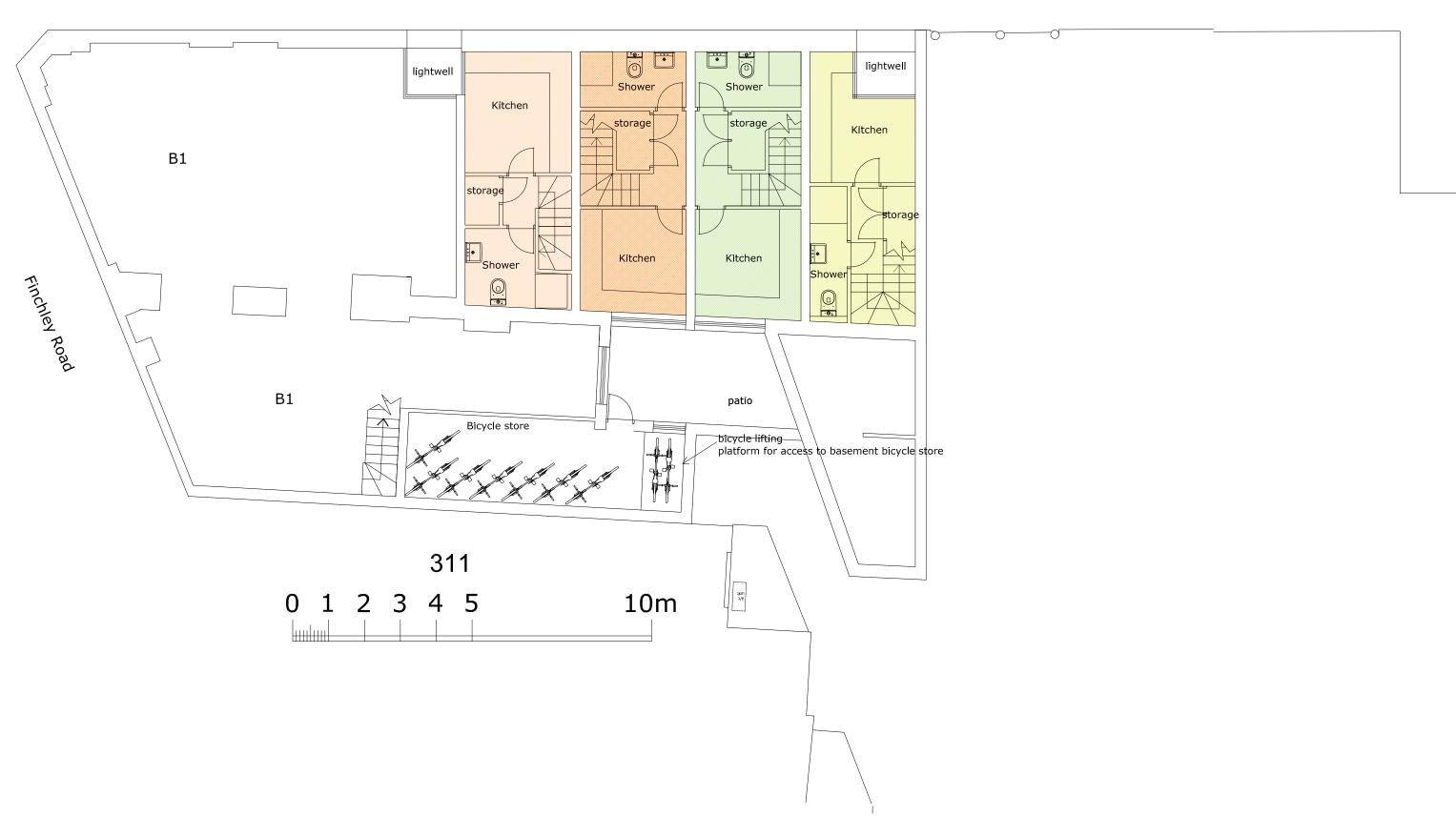
307&309 Finchley Road, London NW3 - Proposed Basement Floor Plan
