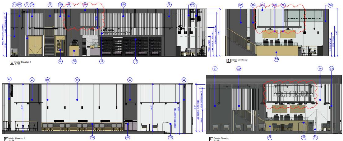
Figure 4: Proposed suspended ceiling details and fixtures
