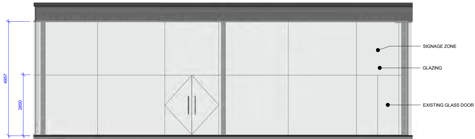
1 EXISTING FRONT ELEVATION 1:100
