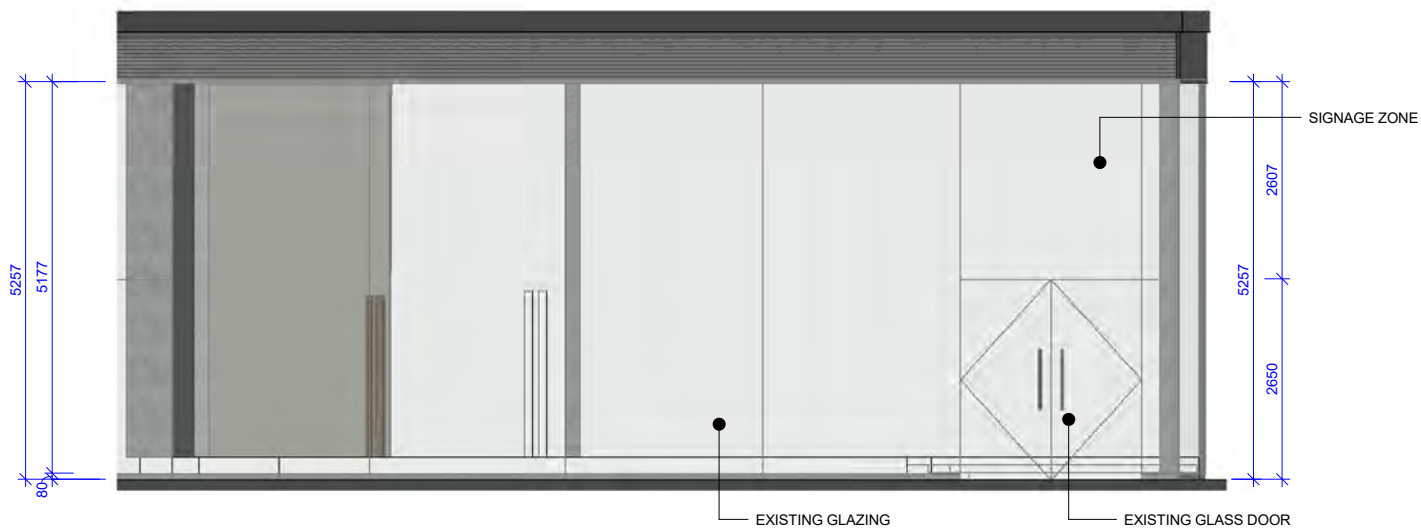
3 EXISTING REAR ELEVATION 1:100
