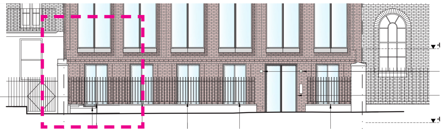
Proposed Part Elevation showing extended railings
