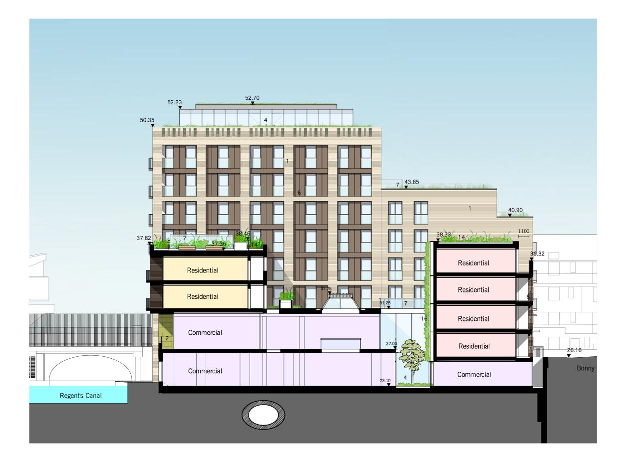
CSC3/S106 **Proposed Section DD** (Block C & Block A)
