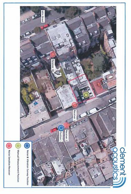
sensitive receivers 12764-SP1 Indicative site plan indicating noise and vibration monitoring positions and nearest noise
