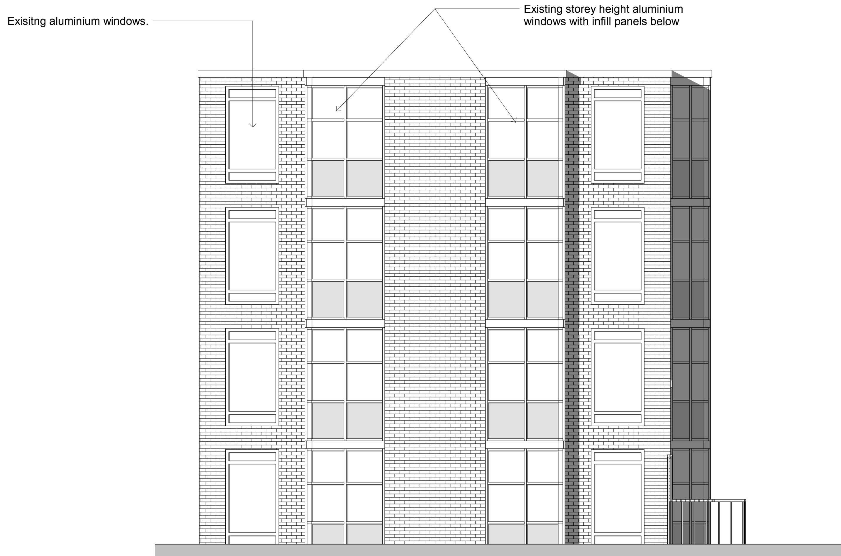
1 Existing North Elevation 1 : 50
