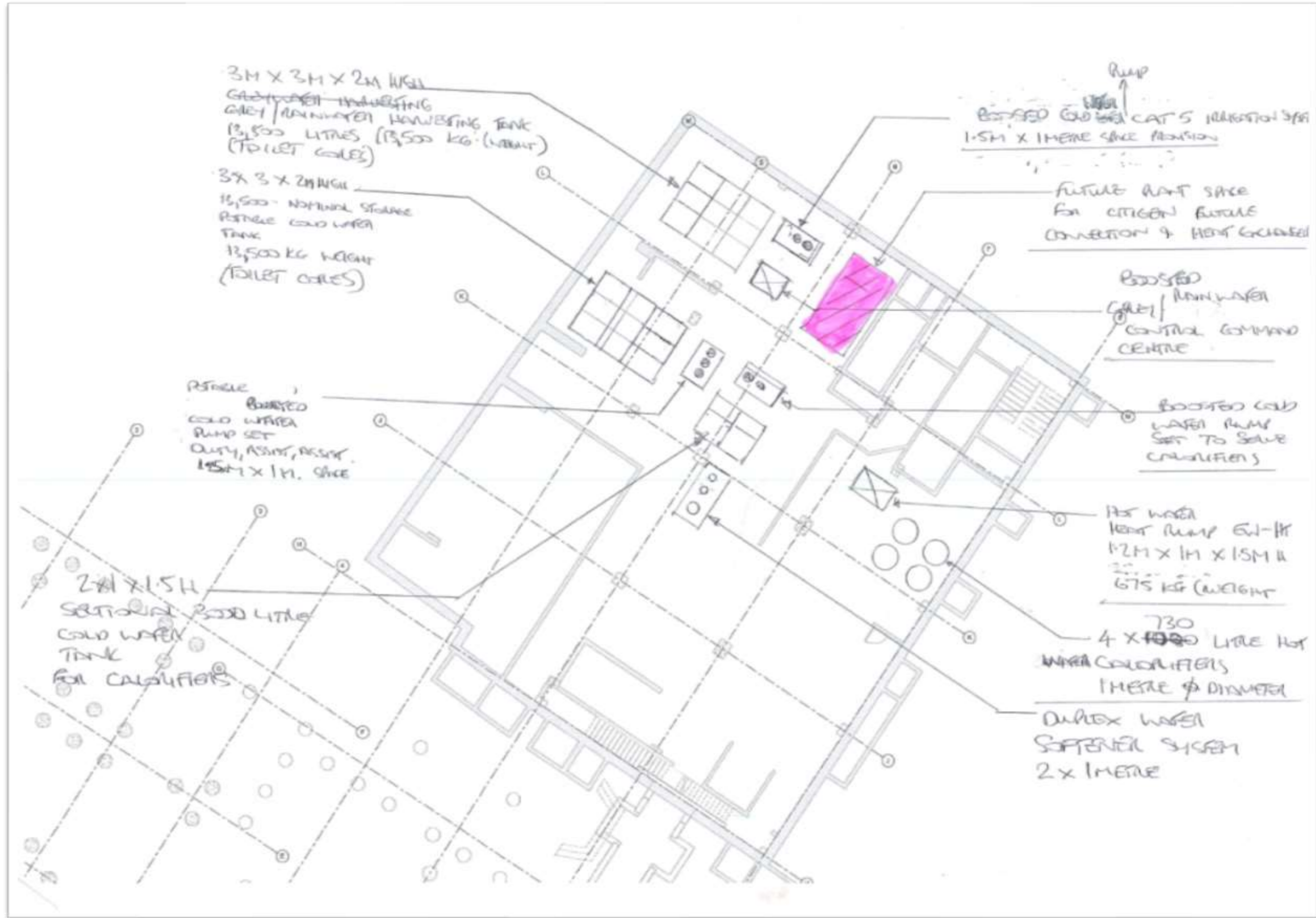
Figure 18. Sketch showing location of plant space for heat exchangers / capped connections for future connection to heat network (e.g Citigen)
