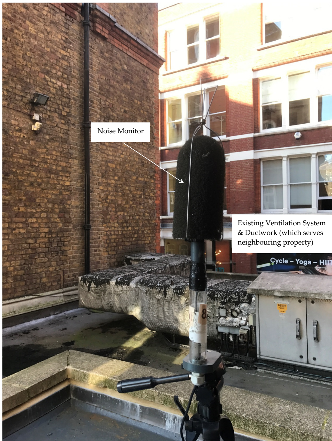
Figure A.2: Noise Monitoring Equipment at rear of 12 Earlham Street
