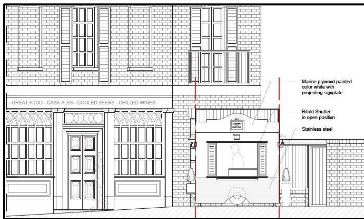
Fig. 3: Proposed replacement kiosk
