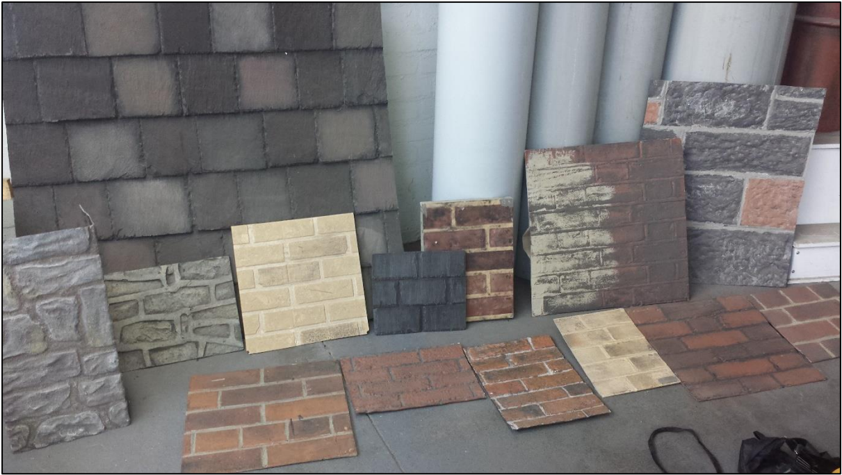
Figure 1b: Examples of GRP reproductions – stone, slate, brick
