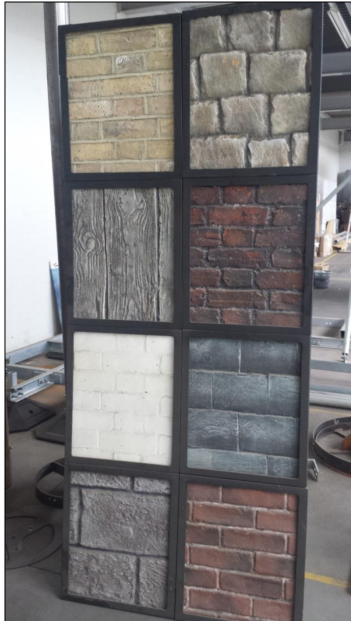
Figure 1a: Examples of GRP reproductions – brick, stone, timber, slate
