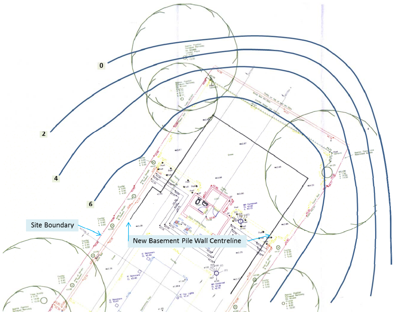
Figure 3: Northern half of Site: Contours of ground settlement arising after basement excavation (in mm)
