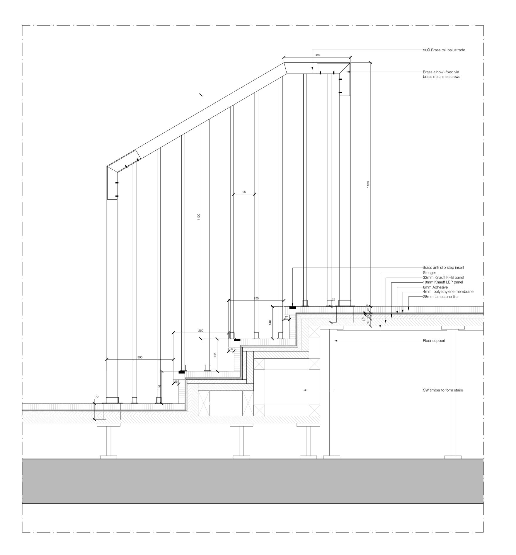
Detail E. Typical stairs detail with rods Scale 1:5
