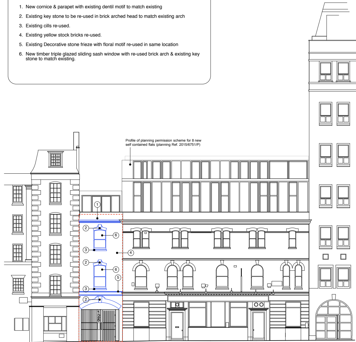
Proposed Clerkenwell Road Elevation - Option 1: Facade Reinstated With Original Features And windows
