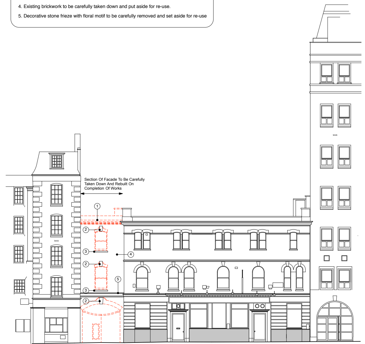
Proposed Demolition Clerkenwell Road Elevation
