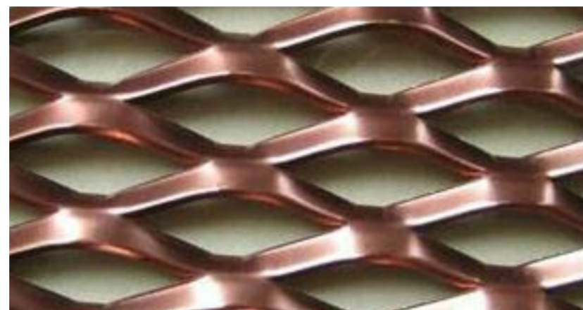
COPPER MESH - ALLOW TO PATINATE AS BELOW
