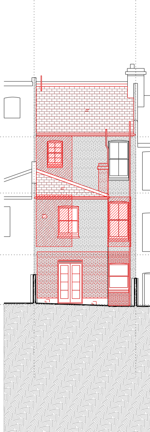
DEMOLITION ELEVATION Y2
