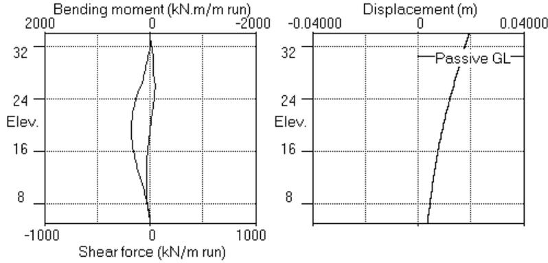
Stage No.2 Excav. to elev. 30.50 on PASSIVE side
