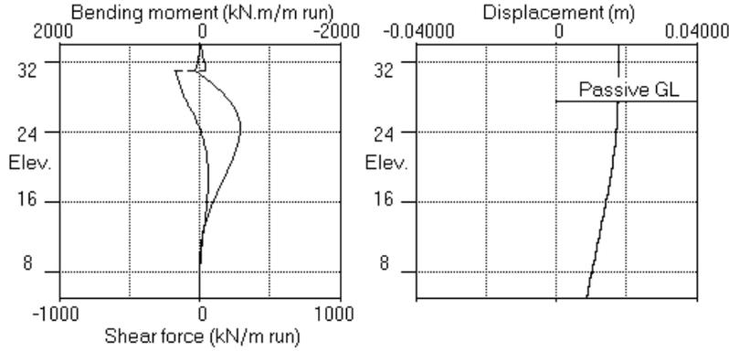
Stage No.3 Excav. to elev. 27.50 on PASSIVE side
