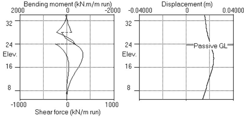
Stage No.12 Change EI of wall to 882019kN.m2/m run
