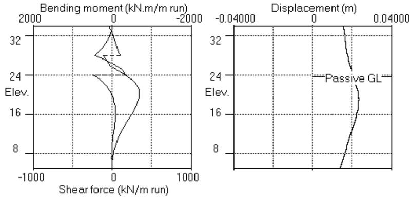
Stage No.11 Change EI of wall to 882019kN.m<sup>2</sup>/m run
