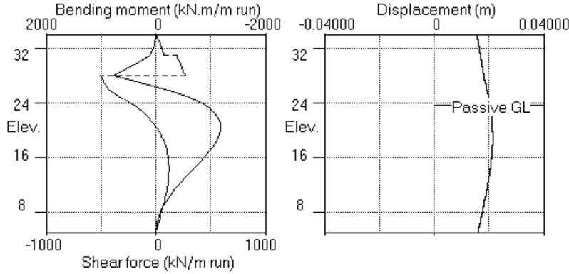
Stage No.6 Excav. to elev. 23.70 on PASSIVE side
