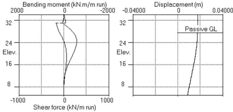
Stage No.4 Excav. to elev. 27.50 on PASSIVE side
