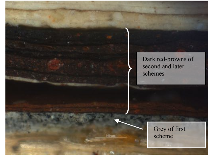
Figure 13: View of early layers in Sample 32B, from skirting on the stairway. The grey of the first scheme is followed by red-brown in the second scheme. Several later schemes employ dark browns.
