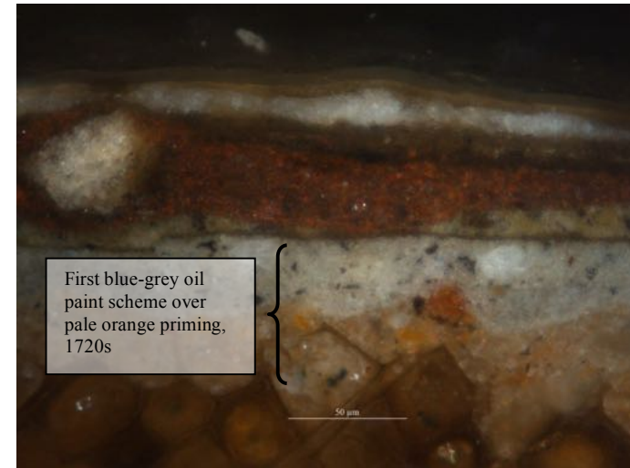
Figure 9: Lower layers of Sample 2, from the skirting of the east wall panelling. The original blue-grey scheme is here applied above a pale orange priming layer.
