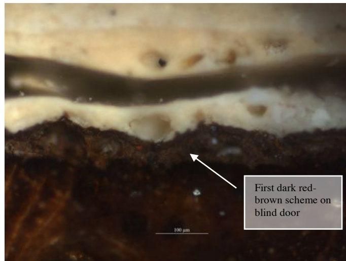
Figure 15: Lower paint layers from Sample 36, on the blind door on the west side, showing the dark brown first scheme applied to the wood surface.
