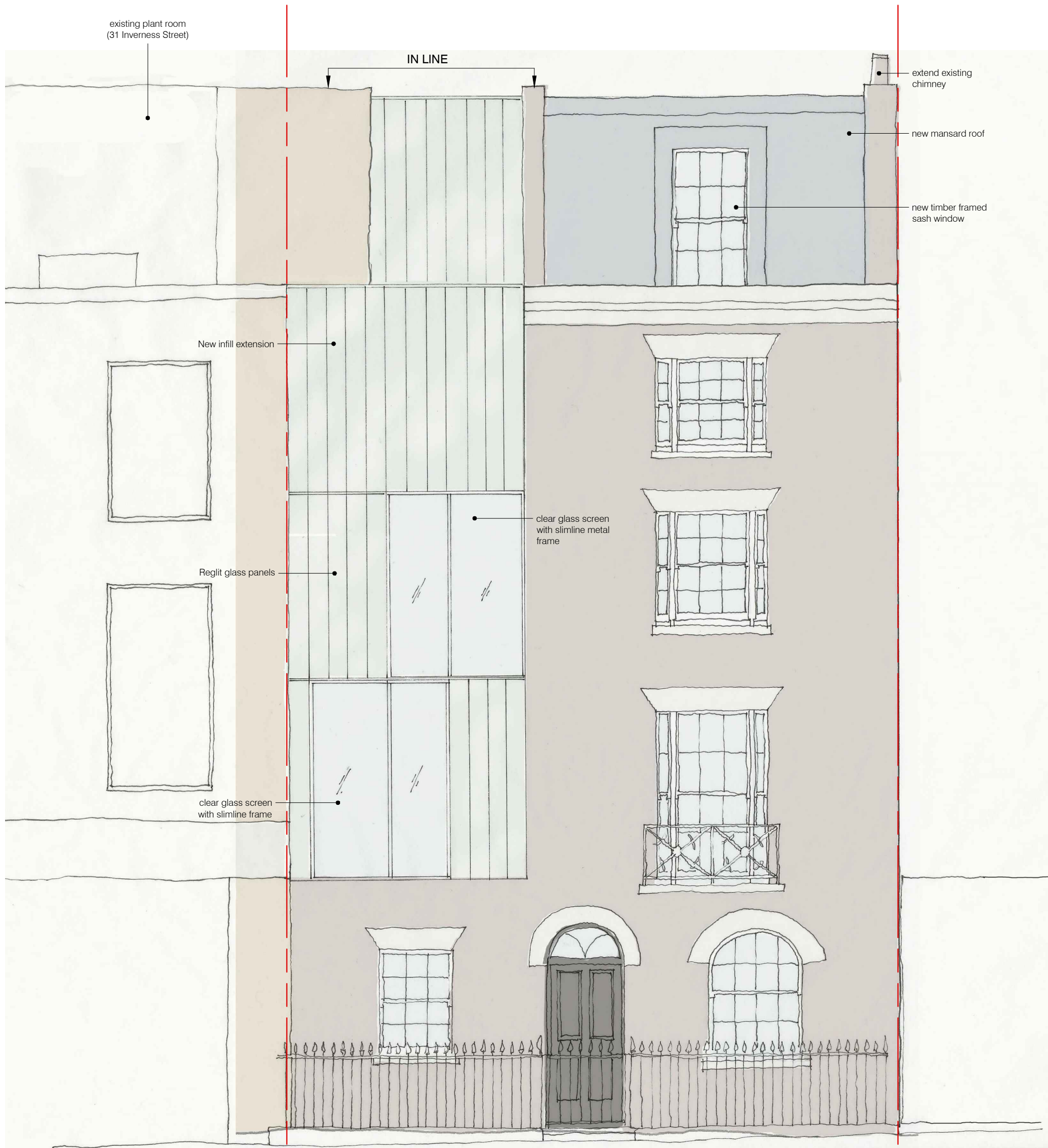
01 PROPOSED FRONT ELEVATION scale 1:50
