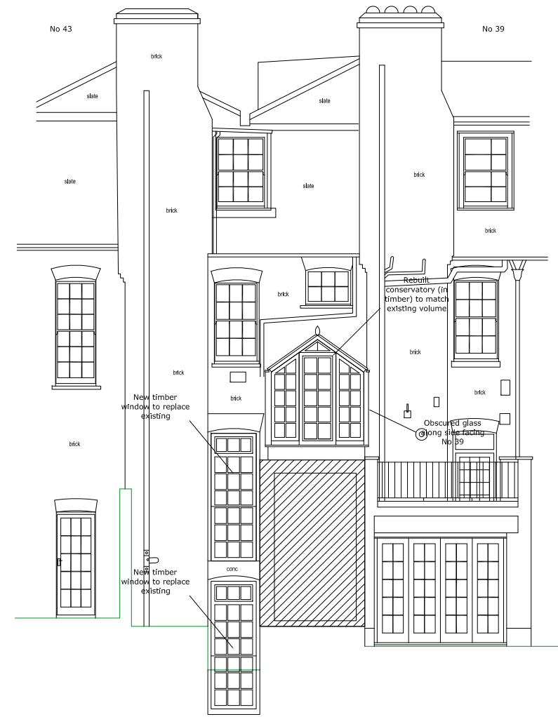
SOUTH-WEST ELEVATION (Rear Courtyard) A.O.D. 23.00m
