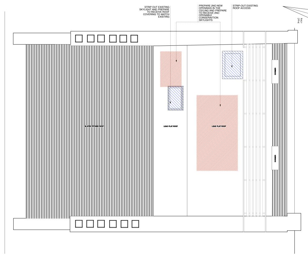
**EXISTING-DEMOLITION ROOF PLAN**
