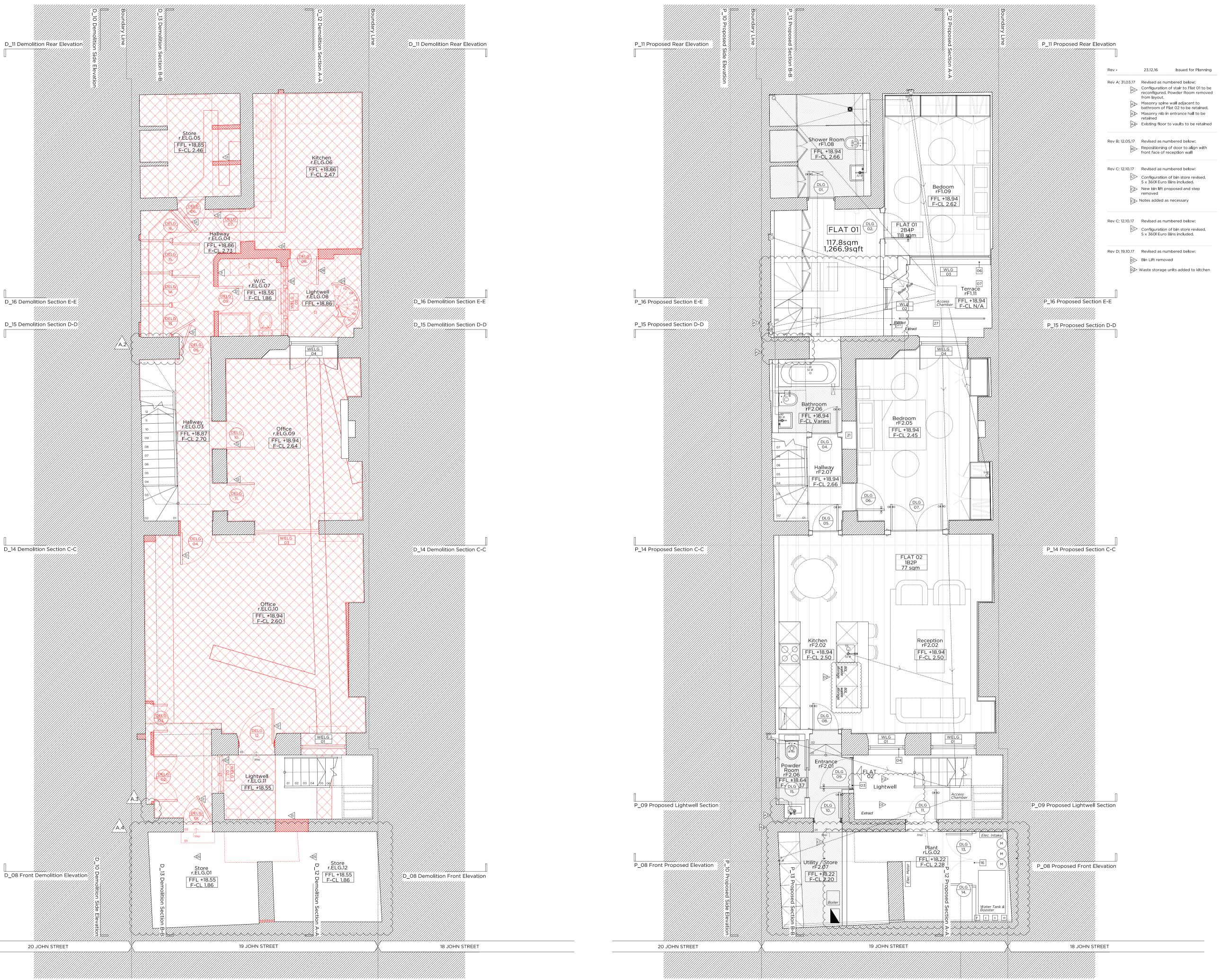
Existing structure / fittings to be removed Hatch denotes area of excavation Existing structure / earth New structure Existing floor finish + substructure to be removed (hatched area) Line denotes removal of existing fittings General Notes: Elevation Key: 1. Refer to the Door and Window Schedules for a detailed summary of the proposal for each door and window.
