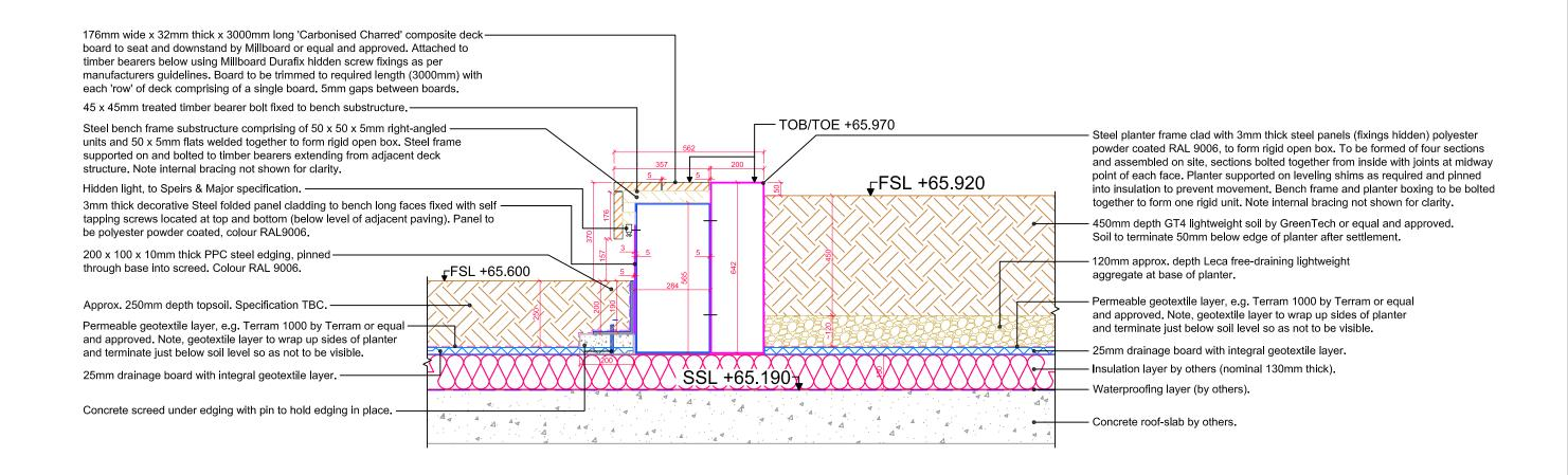
DETAIL 01: SECTION THROUGH LOW PLANTER INTERFACE WITH HIGH PLANTER/SEAT
