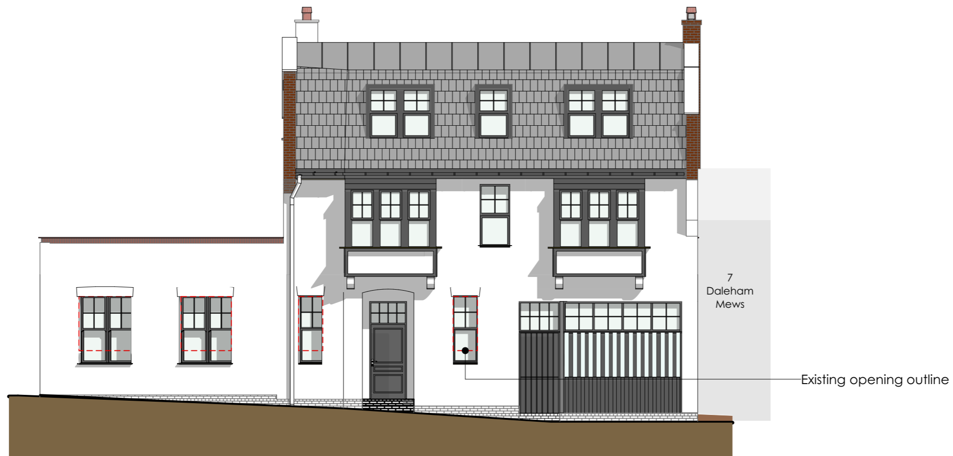
Proposed West Elevation Proposed windows in comparison with existing window openings
