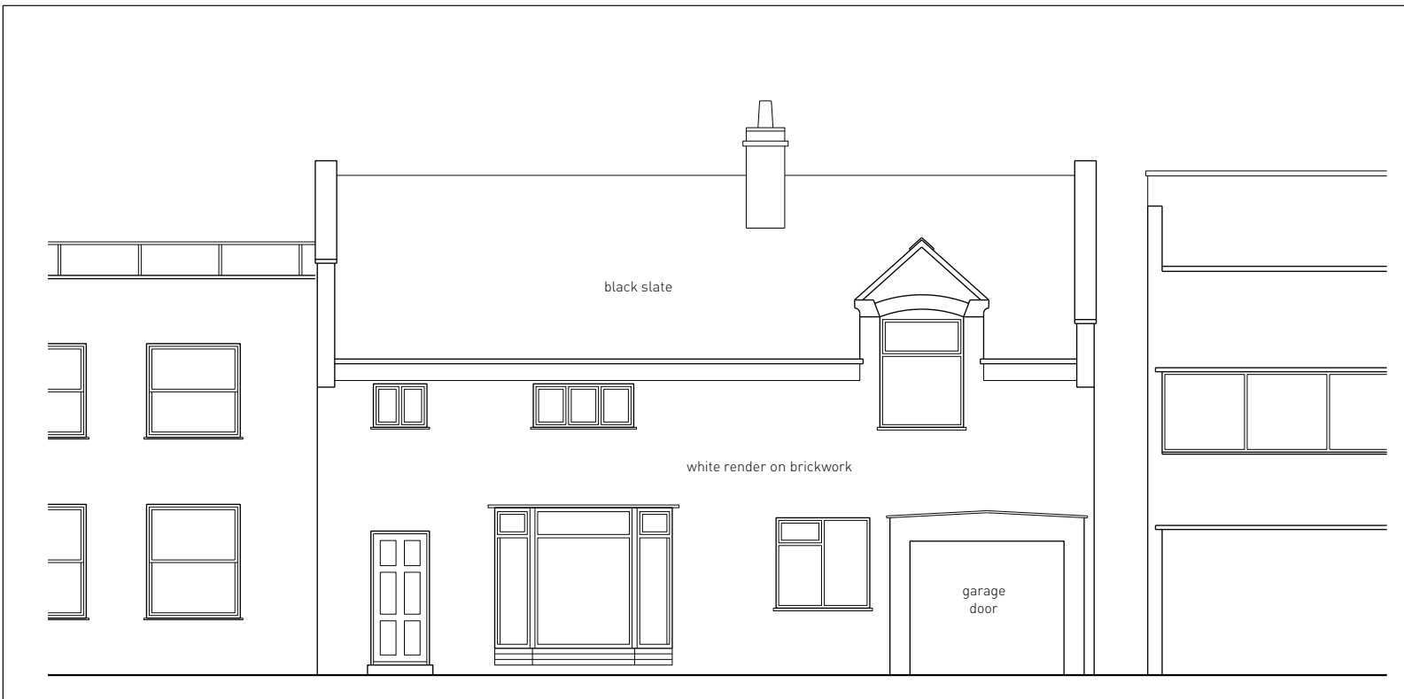
EXISTING FRONT ELEVATION 1:100
