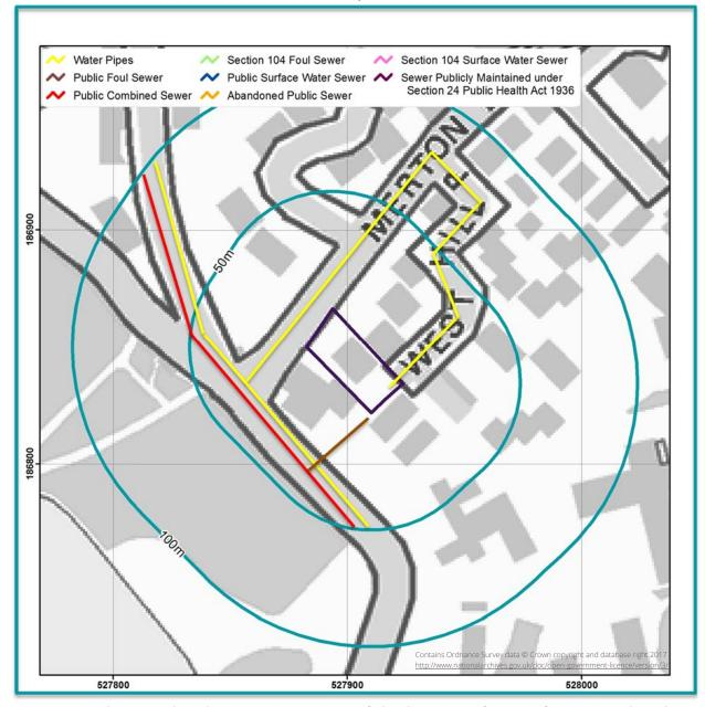
GeoSmart have undertaken an assessment of the location of sewer features within the vicinity of the Site. According to an STL sewer search there is a public combined sewer located within 50m of the Site, according to mapping included within section 8 and Appendix C. Plans provided also shows that the Site is already served by surface water manhole covers located towards the front of the property.
