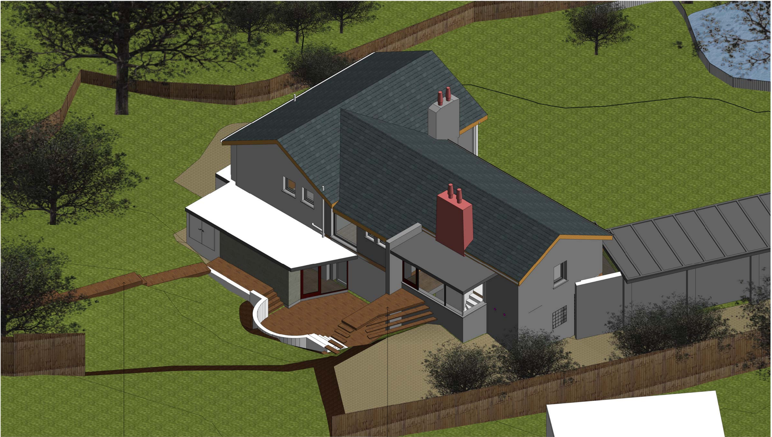
Stepped deck path constructed above ground level
