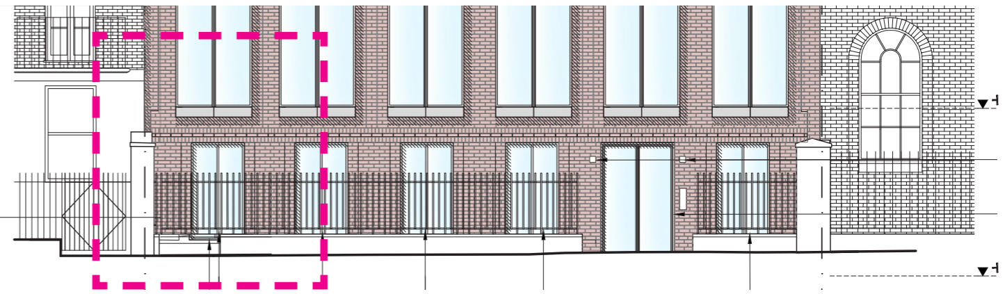
Proposed Part Elevation showing extended railings
