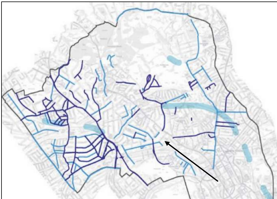
Figure 9. Exact from Figure 15 of the Camden CPG4 showing roads which flooded in 1975 (light blue), in 2002 (dark blue) and 'areas with potential to be at risk from surface water flooding' (wide light blue bands)
