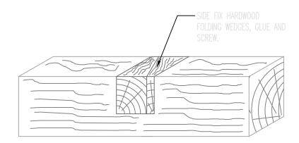
NOTCH REPAIR DETAIL 2
