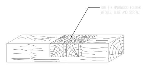
NOTCH REPAIR DETAIL FOR LONG NOTCH
