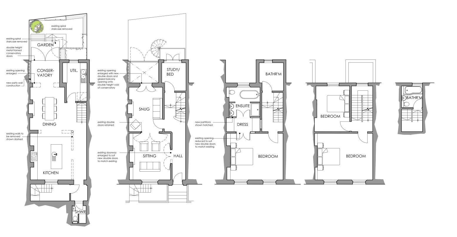
Basement Plan Ground Floor Plan First Floor Plan Second Floor Third Floor Plan
