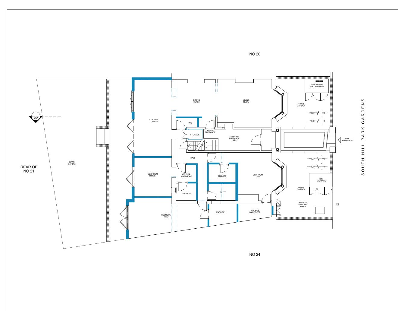
All drawings to be read in conjunction with structural engineer's and service engir Blue linework shows proposed wall
