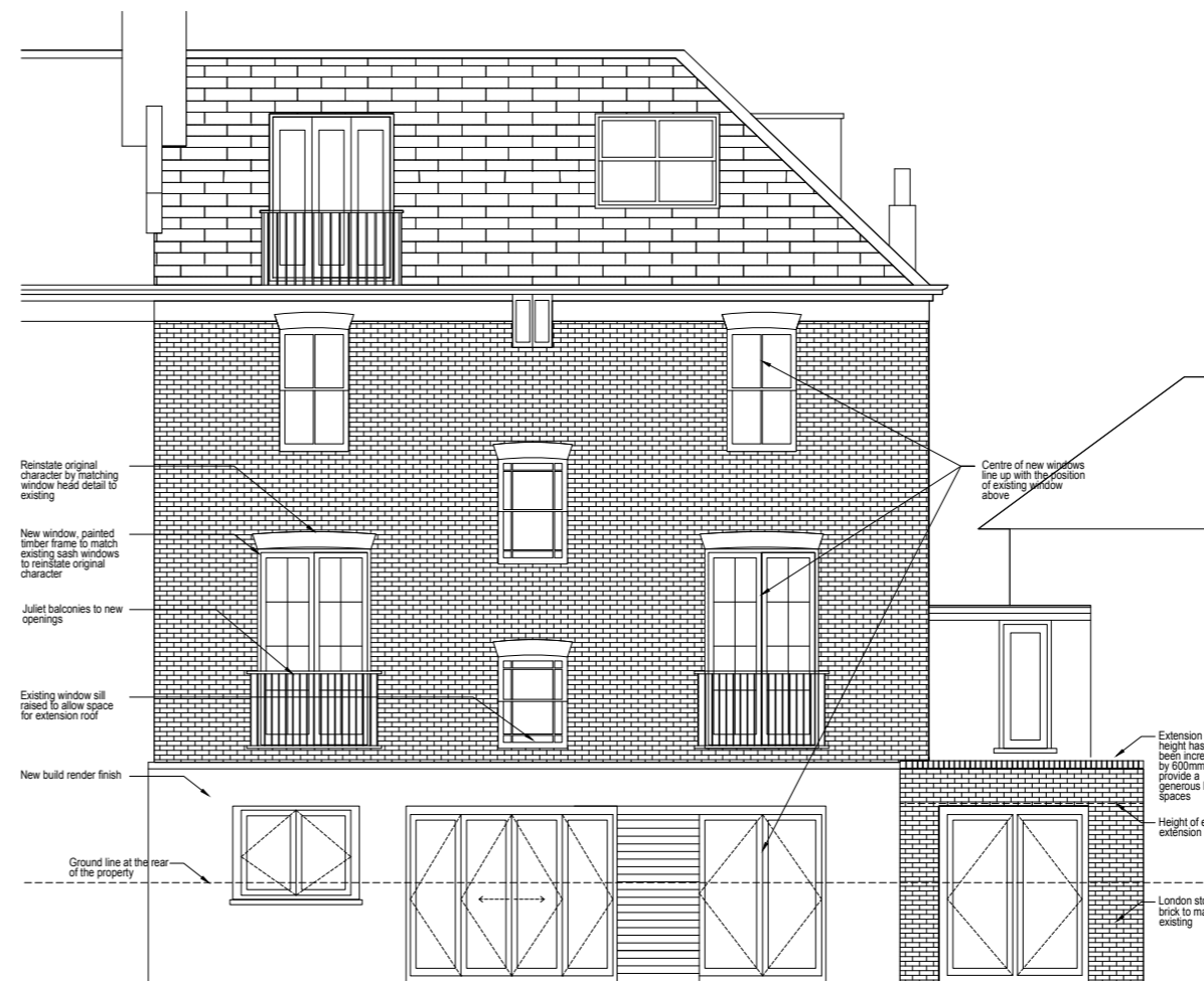
Fig 4.B PROPOSED View of rear elevation, note large windows with juliet balconies to replace four small windows on the right and one sash window on the left and line up with windows above. Sill of the central sash window on first floor raised up.
